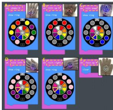
Figure 17. Coding LED bulbs to glow in different colors depending on the direction of wrist movements: (A) on shake; (B) on tilt up; (C) on tilt down; (D) on tilt left; (E) on tilt right; (F) on face up. Captured by the author. (June 11, 2021).
