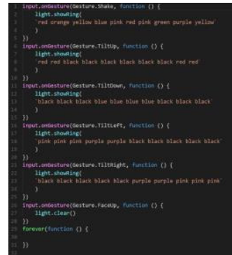
Figure 18. Javascript source of smart gloves with motion sensor. Captured by the author. (June 11, 2021).
